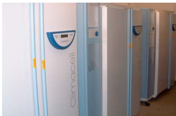
Fig. 3: Climate chamber for storing stability samples
